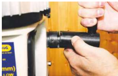
▲ The large plunge handle is easily repositioned to suit the work
